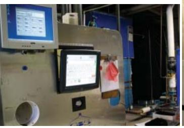
The soil station has an RFID antenna beneath the sorting table to read the chips before they are sent to bins to await washing.
